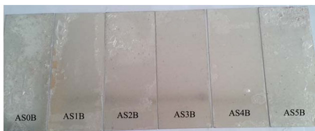
Figure 6. Digital photo of coatings after 3 months at room temperature (base: tin plate). [Color figure can be viewed in the online issue, which is available at wileyonlinelibrary.com .]
